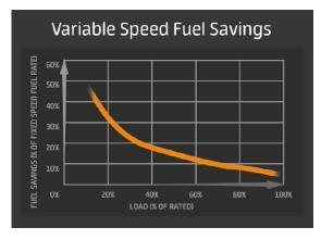
Figure 2: VSG Fuel Savings with Load
