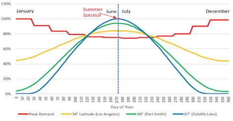
Figure 3: Peak Demand vs Solar Insolation - Courtesy of NTPC
